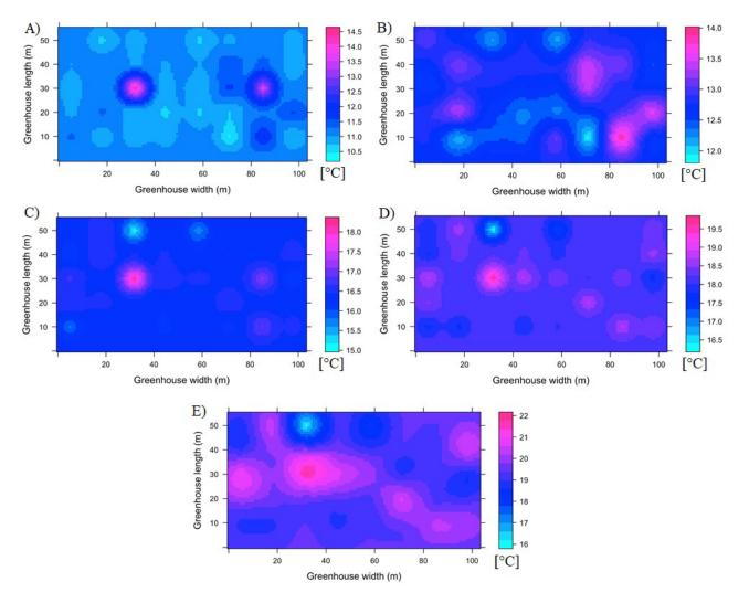
Figure 6. Prediction of temperature [°C] at unsampled points in the greenhouse assessed by radiation groups, (A) group 1, (B) group 2, (C) group 3, (D) group 4 and (E) group 5.
